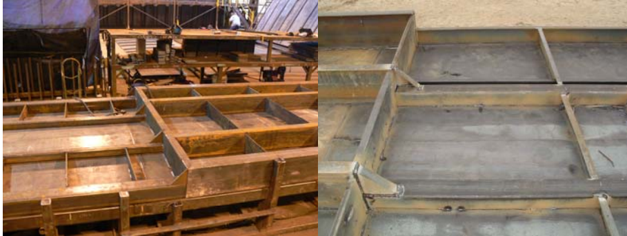
V.E. floor structure: heavy wall tubing rails, maximum bracing, conduit / wiring harness
