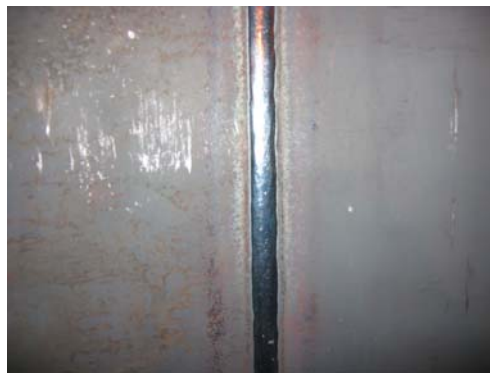
V.E. submerged arc weld utilized on all barrel and wall sections; 100% seam penetration
